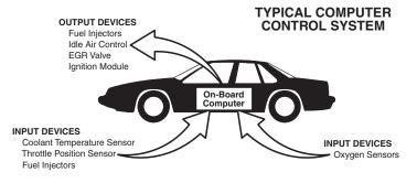
Vehicle operating conditions are constantly changing. The computer continuously makes adjustments or corrections (especially to the air/fuel mixture and spark timing) to keep all the engine systems operating within the preset reference values.
