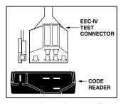
correct test connector for computer service codes use. If you have any questions about the correct connector, please refer to your vehicle's service manual for detailed information.
