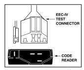
correct test connector for computer service codes use. If you have any questions about the correct connector, please refer to your vehicle's service manual for detailed information.
