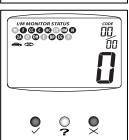
Monitor icons on the LCD display. A **blinking** Monitor icon means the Monitor has not yet run and finished its diagnostic self-testing. All Monitor icons that are **solid** have completed their diagnostic self-testing.
