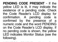
MONITOR STATUS - If the Code Reader's LCD display shows a zero (indicating there are no DTCs present in the vehicle's computer), but the yellow LED is lit, it indicates a "Monitor Has Not Run" status. This means that some of the Monitors on the vehicle have not yet finished their diagnostic self-testing. This condition is confirmed by one or more blinking
